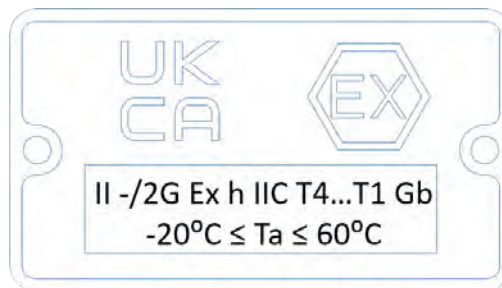
Figure 2: Typical UKCA Ex nameplate
